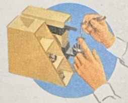
Assembling the electrodes on a special rig.
