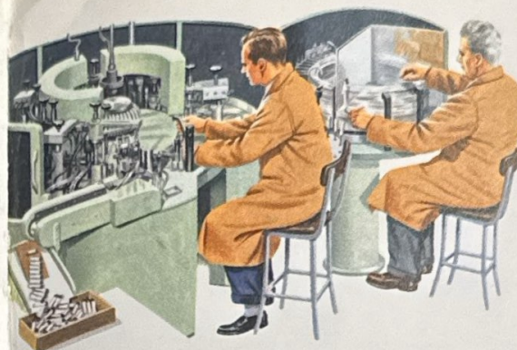
Assembling the electrodes on a special rig.
