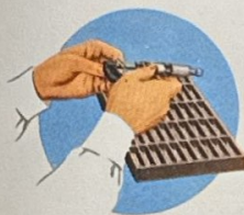
Measuring the size of the grids with a micrometer gauge.
