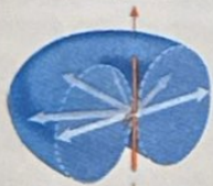
The dipole receives signals from most directions.
