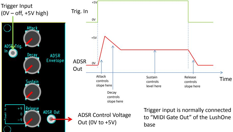
Application Suggestion: Connect ADSR Out to a VCF CV input on the LushOne base for a filter that changes during the note
