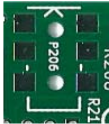
Surface mount pads for jack socket
