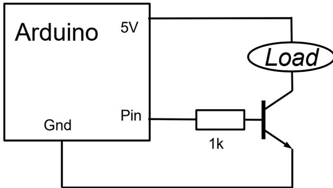
For larger loads, or loads that need a different power supply voltage to the Arduino's 5V the following general circuit can be used. You may need to check the suitability of the transistor. The 2N3704 we are using in the experiments has a maximum capacity of 500mA. To test the current taken by a load connect it to a power supply with a current meter in the path.
