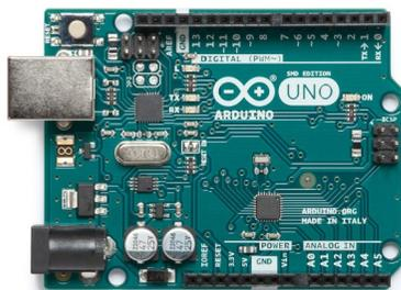
Simplified power supply (automatic selection of USB or external power)
