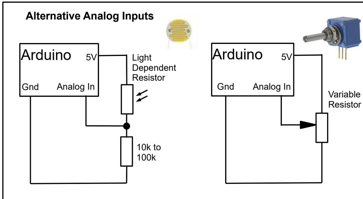
Note: Circuit Diagram only shows the analog input
