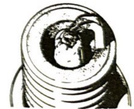
Electrodes burnt away due to wrong heat value or chronic pre-ignition (pink)
