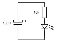
In the first circuit the capacitor charges up with current from the battery. The value of the resistor and the capacitor determine how quickly the charge builds up. As the capacitor charges it develops its own voltage that pushes against the battery. This reduces the flow of current and the LED goes out.
