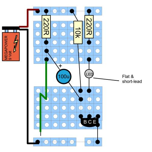
Build the circuit and then try connecting the flying lead to the negative line. The LED should go out momentarily and then relight. Disconnect then reconnect the flying lead to show this is repeatable.
