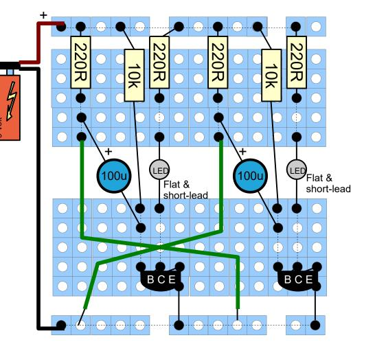
Build the circuit and then try connecting the flying lead to the negative line. The LED should go out momentarily and then relight. Disconnect then reconnect the flying lead to show this is repeatable.
