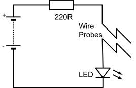
Try touching the ends of the wire probes on to different objects:
