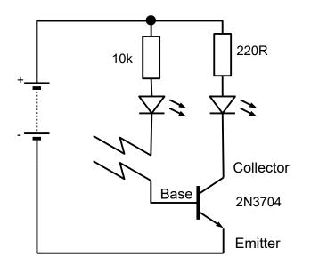
Connect the circuit up as shown and then try applying the probes to various items. Notice the brightness of the two LEDs. You should find the LED in the collector circuit is much brighter than that in the base.
