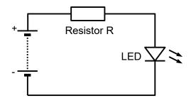
Try using different values of R in this circuit: 100k, 10k, 1k, 220R
